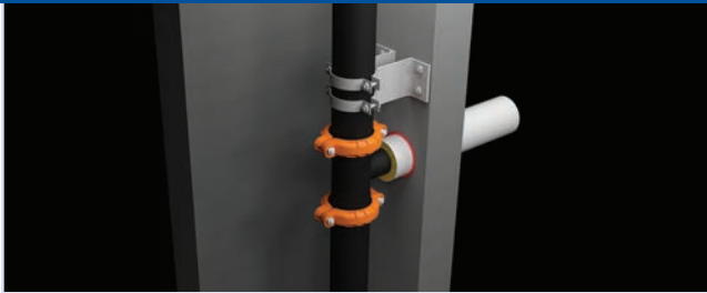
PHOTO 7 Flexible mechanical couplings in vertical piping.
